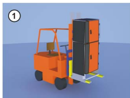
Fig. 6-3: Transportation by fork lift truck
